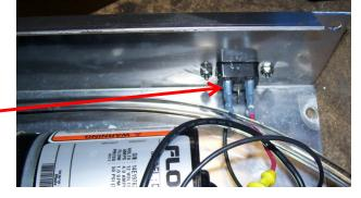
7. From the outside of the base plate, insert the new power receptacle ① through the hole where the old receptacle was. Position the receptacle so the cap is on the right side.
