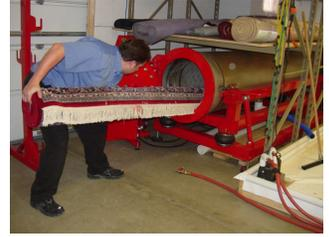
A centrifuge spins water from rugs much the way a washing machine spins to remove water from laundry.
