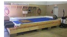
A raised wash pit constructed from lumber and lined with swimming pool liner. The floor is tilted so that water runs off one end.
